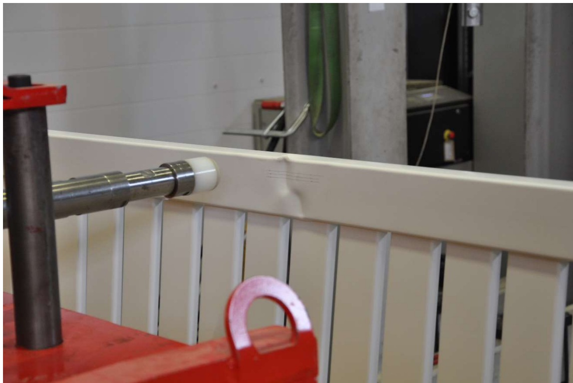
Figure 7. Upper rail damage.
