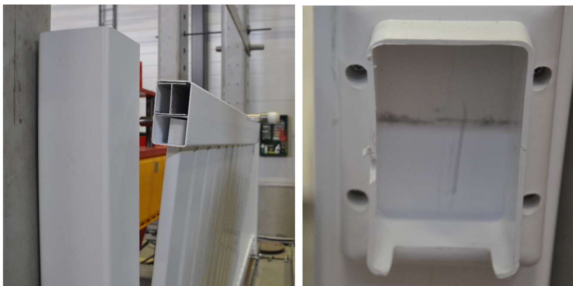
Figure 6. Test 1 barrier structure failure.
