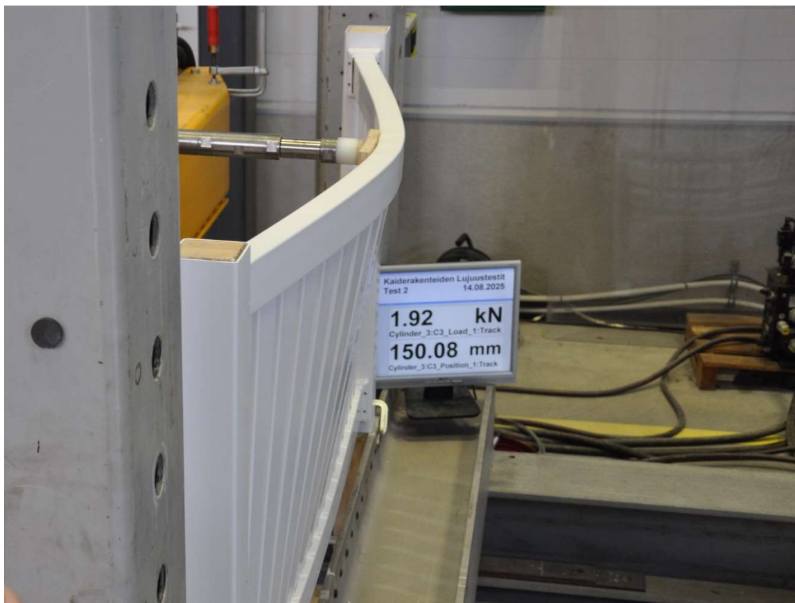
Figure 7. The barrier structure under load during Test 2.
