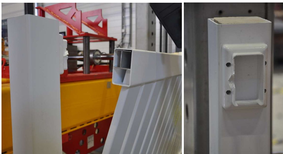
Figure 8. Test 2 barrier structure failure.
