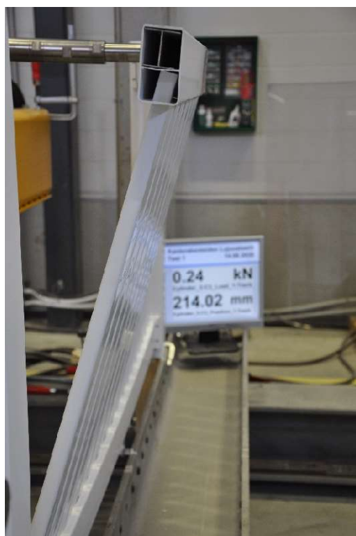
Figure 6. Test 1 barrier structure failure.
