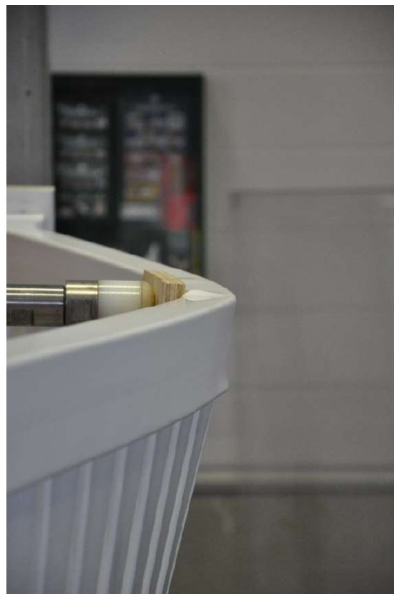
Figure 5. The barrier structure under load and bending of the upper rail during Test 1.
