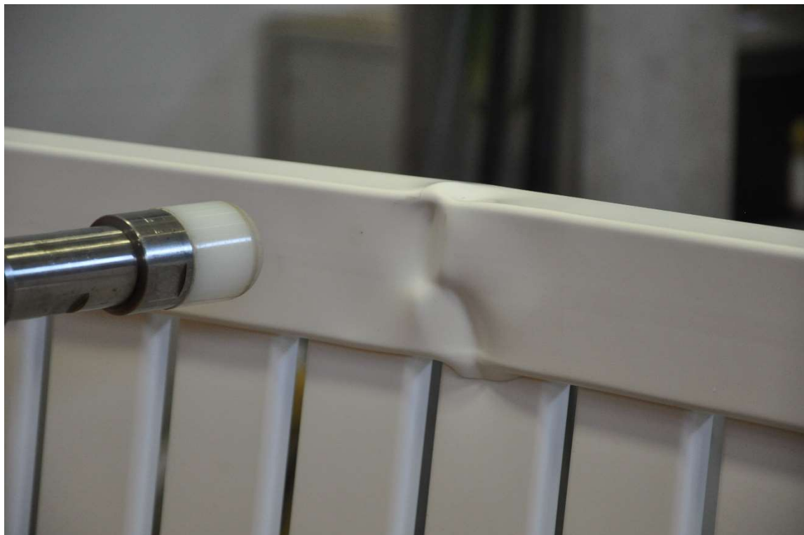
Figure 9. Test 2 upper rail damage.
